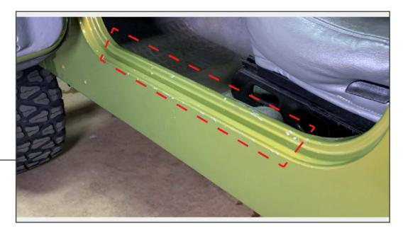
Clean the bottom of the door opening using isopropyl alcohol and a microfiber cloth.
