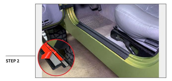
Peel back the film on the double sided tape. Align the door entry guard to the vehicle, then firmly apply pressure to the door sill guard to adhere the guard to the vehicle. Repeat procedure to the opposite side.
