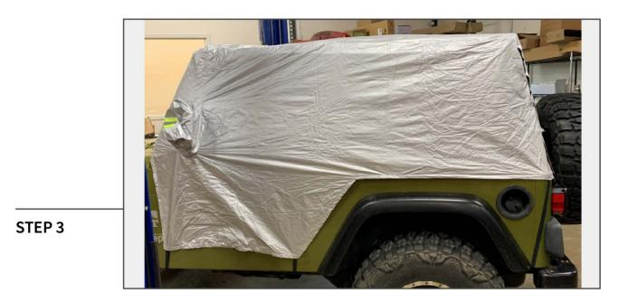
Pull the cab cover over the entire cab. Pull the sides over the mirrors and down the doors. Make sure the cab cover is even on all sides.
