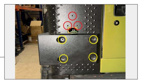
Plug in and reinstall the tail light to the vehicle using original hardware. Using the (4) license plate bracket bolts, secure the armor to the vehicle.
