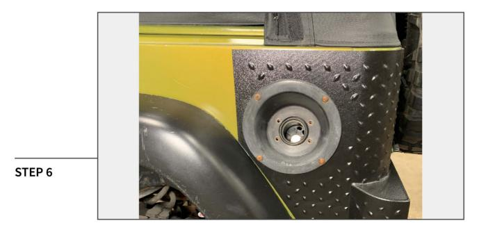
Reinstall the gas cap bezel reusing original hardware.
