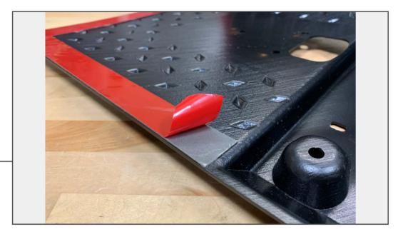
Peel back the film on the provided double sided tape. While aligning the bolt holes on the vehicle with the armor, adhere the armor to the vehicle.
