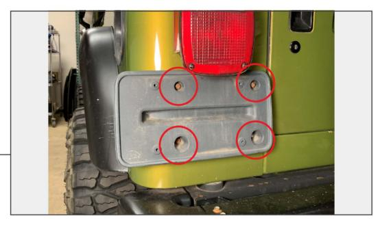
Remove the license plate from the vehicle. Remove (4) 10mm bolts to remove the license plate bracket from the vehicle.
