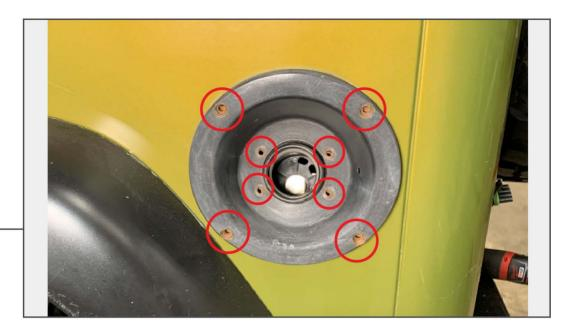
Remove the gas cap from the vehicle. Remove (8) Phillips screws from the gas cap bezel. Remove bezel from vehicle.
