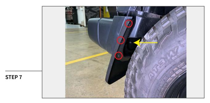
Once drilled, reinstall the mud guard to the vehicle using the 8mm bolt. Use the provided (3) plastic rivets to secure the side of the mud guard to the bumper.
