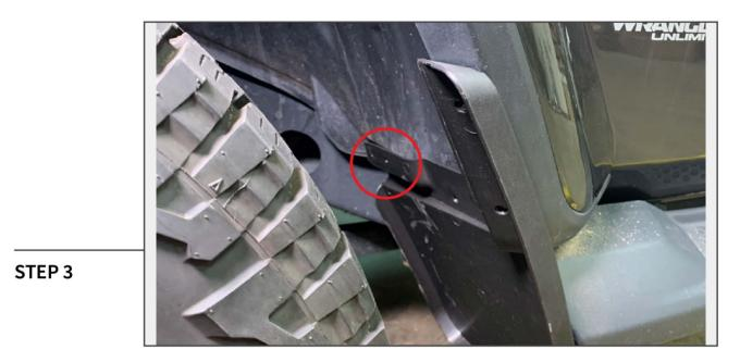
Once the mud guard is secured with the (4) plastic rivets, use the mud guard as a template and drill a 1/4" hole through the fender liner. Install (1) plastic rivet through the mud guard into the fender liner.
