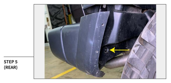
Remove (1) 8mm bolt from the rear fender liner.
