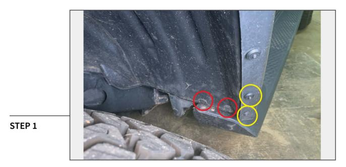
Using a panel removal tool, remove the (2) plastic push clips in the fender liner. Cut the (2) plastic rivets off of the fender flare trim.
