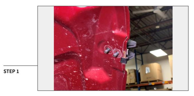
Open the hood on the vehicle. Remove (2) 10mm nuts to remove the hood latch from the vehicle.
