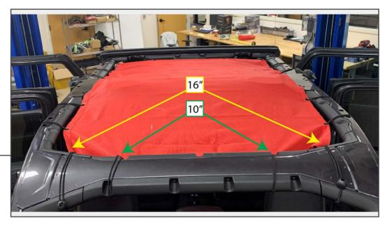
Use (2) 10" elastic bands and (2) 16" elastic bands to secure the mesh top to the rear of the vehicle.
