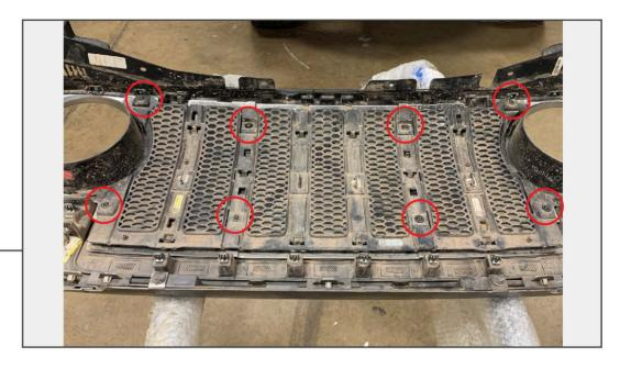
Remove the (8) T-20 Torx bolts from the back of the grille.
