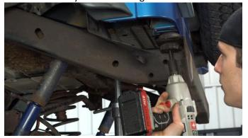
Remove the rear cross member. (If you are not replacing it with the rear frame sections you will need to carefully cut it away from the frame rails.)
