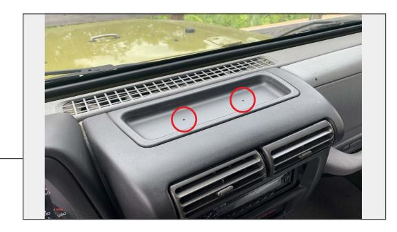
Remove the rubber dash pad, and remove (2) Phillips screws from the dashboard.
