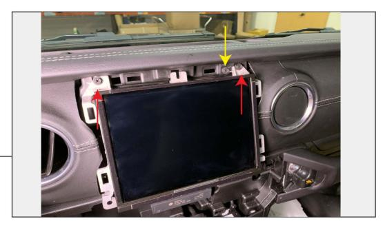
Remove the (2) Phillips screws to release the touch screen from the dashboard. Allow the touch screen to hang. Remove (1) Phillips screw from the dash pad.
