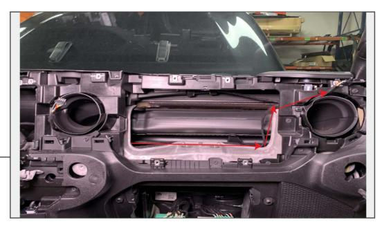
Route the wiring harness to the passenger side outer duct. Be sure to route the wiring harness neatly to prevent interference with the airbag.
