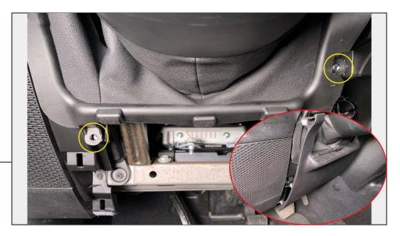
Remove plastic panel below steering wheel using a panel removal tool. Then remove (2) Phillips screws to release the bezel around the steering wheel.
