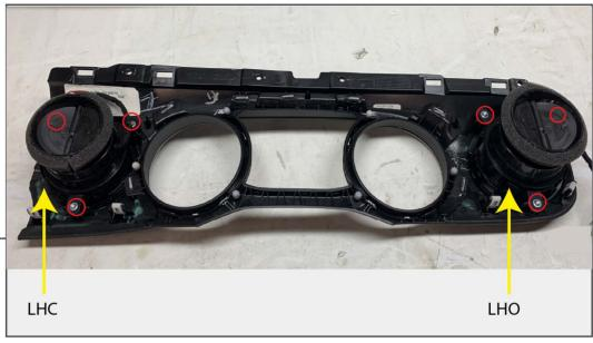
Remove (3) T15 Torx screws securing the each vent to the airbag assembly. Lightly pry back on the plastic mounting tabs to release each vent from the airbag assembly. Do not mix up the vent locations.
