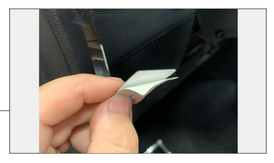
Route power switch to desired location, then using provided double sided tape, adhere to clean surface area of the dashboard.
