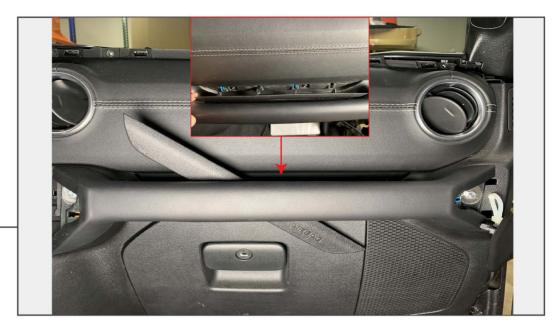
Remove the side cap from the grab handle. Remove (2) 10mm bolts to remove handle from dashboard. Remove from vehicle. Release the airbag trim panel using a panel removal tool.
