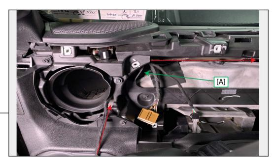
Beginning with the passenger side of the wiring harness, route the harness throughout the dashboard. Store the power module at the marked location [A].
