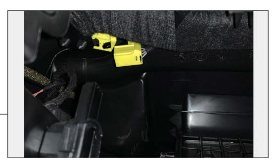
Along the left hand side of the dashboard behind the glove box location, unplug the airbag connector by pushing down on the top of the connector. Remove airbag assembly from vehicle.
