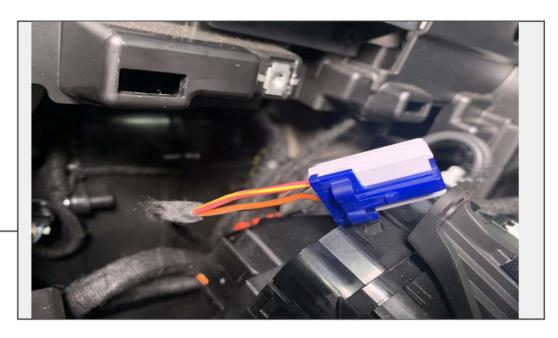
Carefully peeling back the insulation on the cigarette lighter connector, splice into the Red/Yellow wire with the Orange wire in the provided wiring harness. Cut the provided Orange power wire on the provided wire harness to length if it is too long.
