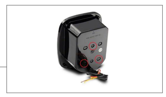
Use a punch and a hammer and tap out the appropriate mounting bolt holes in the tail light housing.
