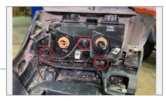
Remove (3) T30 Torx bolts from fender skeleton. Remove fender skeleton away from inner fender.
