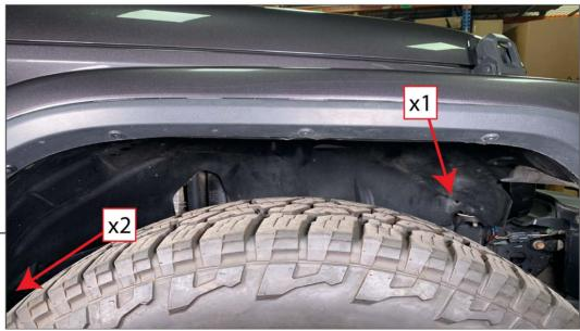
Remove the (3) push clips from the fender liner using a panel removal tool.
