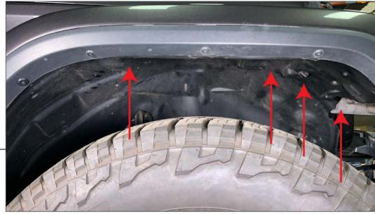
Remove (4) 10mm bolts inside the fender well.
