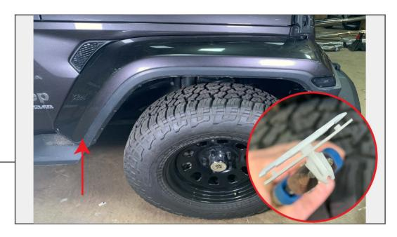
Using pliers, depress the white fender clips while pulling the fender away from the vehicle. Start at the bottom of the fender closest to the doors.
