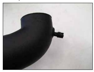
13. Remove the inlet air temperature sensor from the factory intake tube. Remove the O-ring from the sensor and then install the sensor into the K&N® intake tube using the provided grommet.
