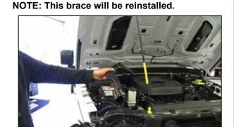
8. Remove the two bolts that secure the fresh air duct to the core support and then remove the duct from the vehicle.
