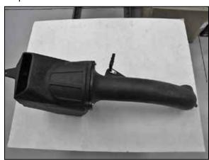
15. Install the intake tube assembly into the K&N<sup>®</sup> air filter housing and secure with the provided hardware.
