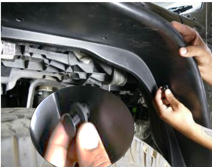
Step 10 Adjust the flare until the hole in the flare is centered over the holes in the L brackets. Insert supplied push rivet (L) onto all 5 positions in the inner bottom part of the front fender flare (A) as shown above. Repeat all steps above for other side of Jeep.
