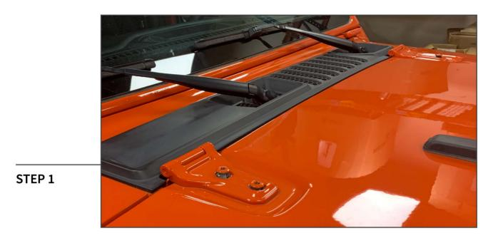
Remove the (2) T50 Torx hood hinge bolts per hinge.
