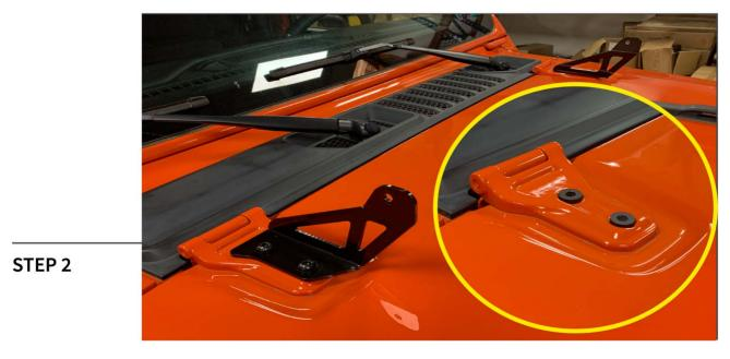
Install the (2) hood mount spacers on each hinge, then loosely install the hood mount bracket onto the hinges using the (2) provided T40 Torx bolts per hinge.
