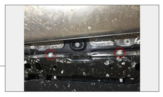
From directly center under the vehicle, locate and remove the (2) 16mm bolts supporting the center of the bumper.
