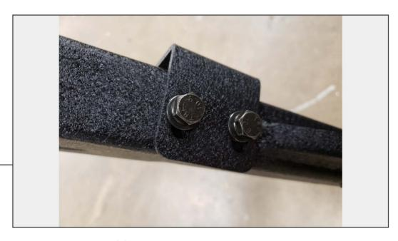
Install the carrier bump stops using the (4)  $M10 \times 1.50 \times 30$ mm bolts. With the carrier latched to the bumper, tighten the brackets so that the brackets are making contact with the rubber bumpers on the tailgate.
