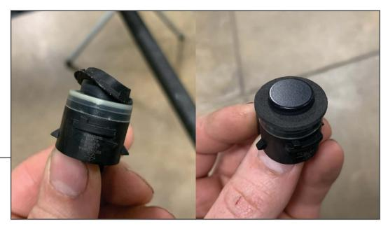
**Optional:** If equipped with proximity sensors, remove the sensors from the bumper. Then remove the rubber gasket from the sensor. Prepare the sensor for re-installation by applying the supplied foam ring to the sensor. Then reference steps 10-12 for the mounting options.
