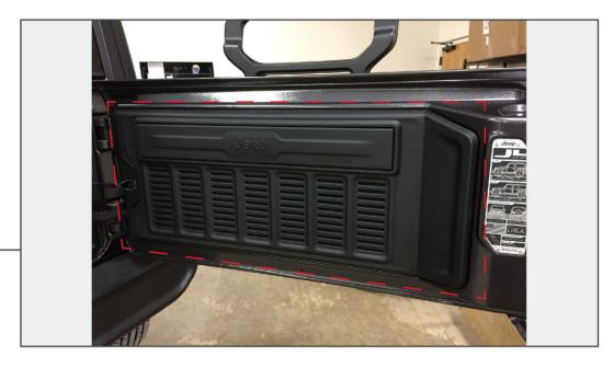
Using a trim panel removal tool, carefully pry the plastic tailgate cover from the tailgate. Remove the cover.
