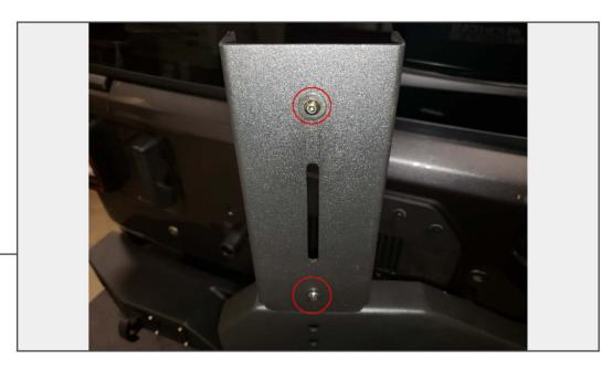
Install the upper bracket to the lower bracket using the (2) M6  $\times$  1.00  $\times$  25mm bolts, flat washers, and lock nuts.
