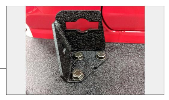
Install the latch bracket to the rear bumper by using the (3) M10 x 40mm bolts, (6) flat washers, and (3) lock nuts.
