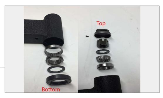
Install the larger bearing and race into the bottom of the tire carrier, and the smaller bearing and race on the top of the tire carrier. Make sure to pack the bearing with grease before installation. Then use the small washer for the top and the larger washer for the bottom. Install the seal on the bottom of the tire carrier. Also use a small amount of grease for the seal.
