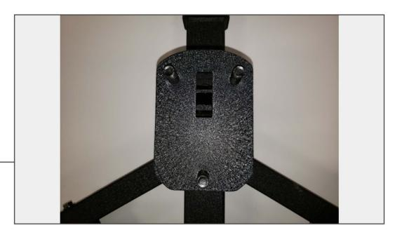
Install the (1) Tire Carrier Mounting Hub to the tire carrier base by using (2) M12 x 1.75 x 80mm bolts, (4) flat washers, and (2) lock nuts. Then install the (1) M12 x  $1.75 \times 30$ mm bolt to lock the hub in place.
