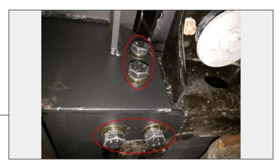
Install the bumper to the vehicle using the (4) 9/16 bolts, flat washers, and lock washers on each side. Torque to 40 ft-lbs.
