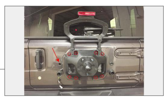
Carefully remove the wiring and grommet from the vehicle. Locate, and remove the (8) 13mm bolts holding the tire carrier secure. Remove tire carrier.
