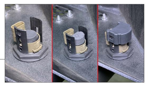
**Optional Sensor Mounting:** Place the round foam on the back of the sensor. Press the sensor into the bumper. Then clip the retaining plate onto the bumper to hold the sensor in place.
