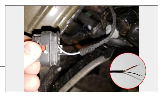
Insert the (2) license plate light LEDs through the license plate bracket and attach with the supplied nuts and washers. Next, splice the Red 12v+ wire from the license plate led harness into the White power wire of the factory bumper harness, and the Black 12v- wire from the license plate led harness to the Black wire on the factory bumper harness connector. Test to ensure proper function.
