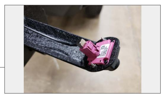
Remove the factory rear backup camera from the factory tire carrier using a T-9 Torx bit. Install the camera to the new bracket using the (3) M2 screws, washers, and nuts.
