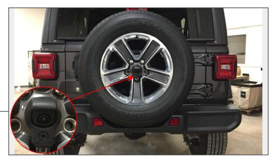
Locate the T-40 Torx lock screw on the camera cover, and turn it counter clockwise to unlock. Remove the camera cover by pulling away from the vehicle. Then, remove the spare tire.
