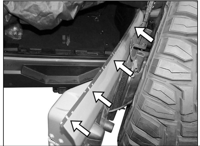
(Fig 25) Apply (1) strip of Double Sided Tape to outside of tailgate, DO NOT REMOVE OUTER BACKING TAPE! Repeat to apply (1) strip of Tape to inside of tailgate
