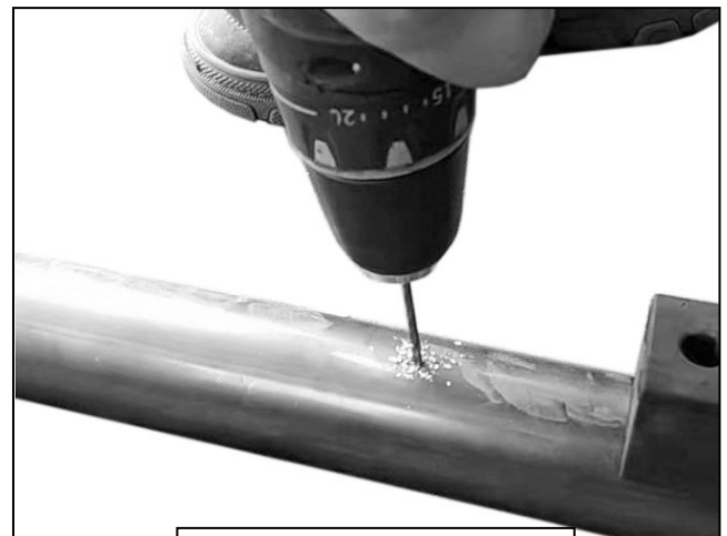
(Fig 22) Drill 1/8" pilot hole
