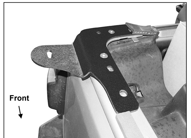
(Fig 12) Passenger/right Mounting Bracket installed
