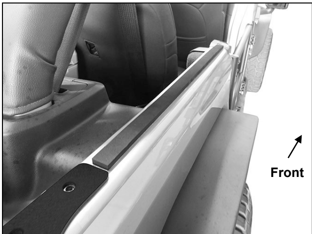
(Fig 14) Install Foam Seal in original location
