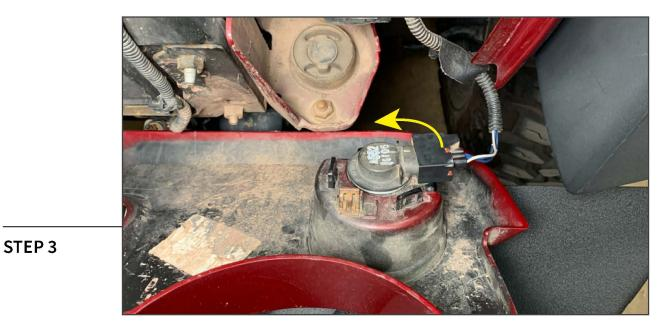
Twist the turn signal socket to remove the turn signal bulbs from the grille. Remove the grille from the vehicle.
