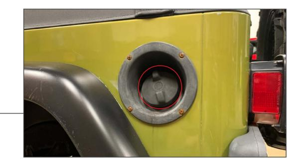
Begin by removing the fuel filler cap.
