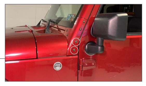
Locate and remove the (2) T40 Torx screws at the base of the windshield.
