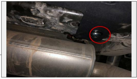
Install (1) M10 Allen bolt and (1) M10 washer on each side underneath the bumper support.
