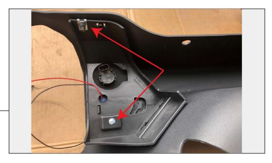
Install parking sensors into the bumper. Attach the bumper inserts for the side parking sensors by using (1) M8 bolt and (1) Phillips screw per side.
