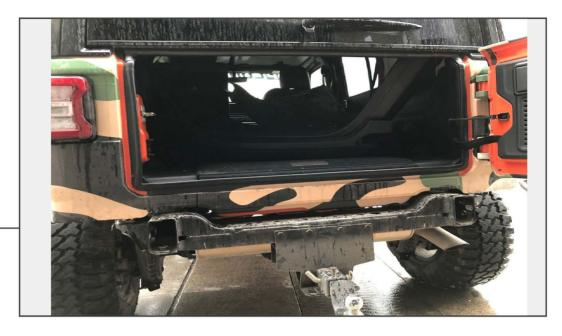
Remove rear bumper from vehicle, exposing the vehicles frame.
