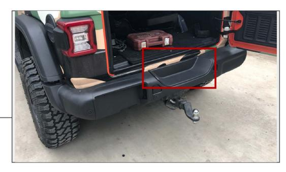
Install the plastic cover over the middle of the bumper. Installation is now complete.
