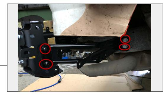
Install (2) original bumper bolts into the support bracket, then once bumper is installed, install (2) M8 allen bolts and (2) M8 washers into the bumper.
