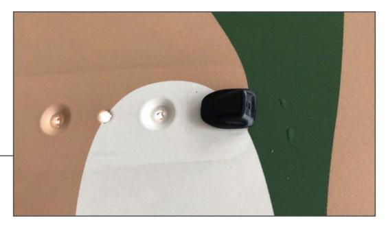
Remove the (2) windshield washer nozzles and transfer them to the new hood.
