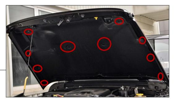
Begin by raising the hood to gain access to the under-hood insulation. Using a panel removal tool, remove the (10) push securing the insulation to the hood. Remove the insulation from the vehicle. Disconnect the windshield washer hose.
