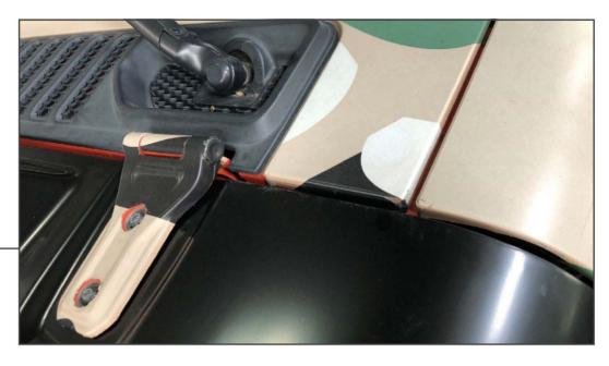
With a helper, install the hood back on the vehicle. Carefully adjust the hood for best fitment. Ensure the gaps are uniform from side to side.
