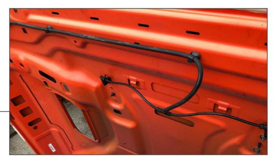
Remove the windshield washer lines from the underside of the hood. Transfer the windshield washer line to the new hood.
