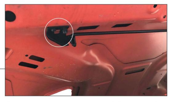
Remove the 10mm bolt securing the hood prop rod to the hood. Transfer the hood prop to the new hood. Reuse the factory hardware.
