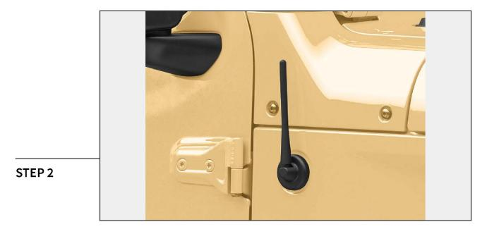
Compare the included threaded adapters to the OEM antenna to find the appropriate adapter. Once the appropriate adapter is found, thread the adapter onto the new antenna until secure.
