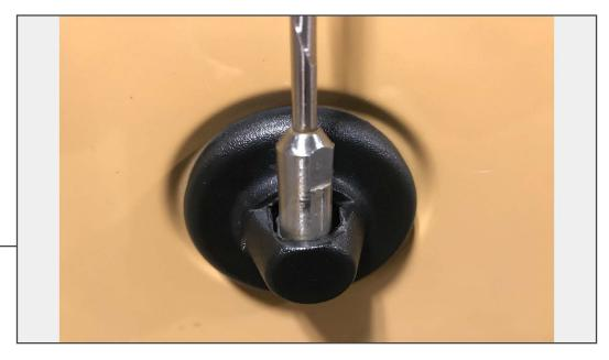
Using a small adjustable wrench, rotate the antenna counter-clock wise to remove it from the vehicle.
