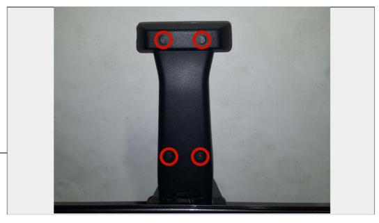
Begin by removing the (4) screws that hold the factory third brake light to the tire carrier. Unplug the wiring harness from the third brake light and remove the third brake light from the vehicle.
