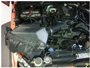
Step 5: Remove your factory IAT sensor from the factory intake tube.
