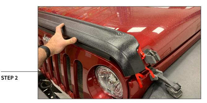
Test fit the part before removing any tape backing. Ensure you are comfortable with where the part fits best on the vehicle.
