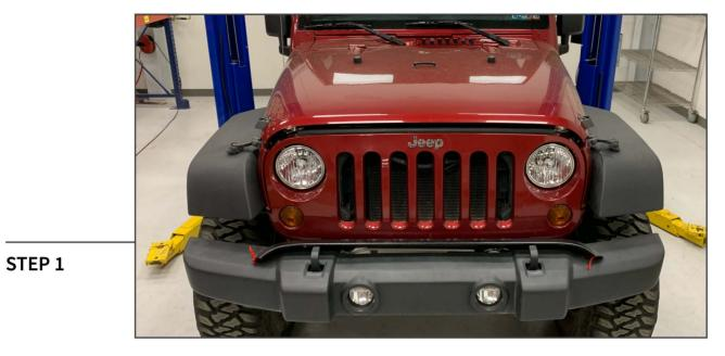
Begin by thoroughly cleaning the front edge of the hood and the top edge of the tailgate using automotive grade soap and water. Allow the vehicle time to dry. \*\*Recommended: Wipe the hood/ tailgate mounting surface with isopropyl alcohol to ensure the cleanest possible surface.
