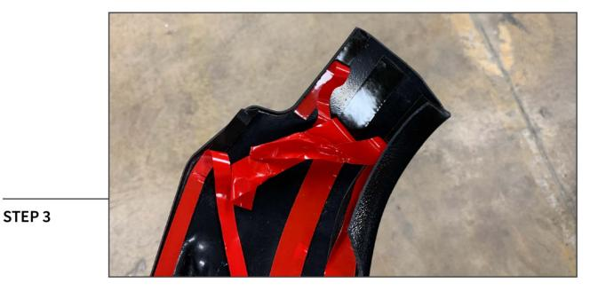
Remove the tape backing and carefully install the part to the vehicle. Apply firm even pressure over taped surfaces to ensure proper adhesion.
