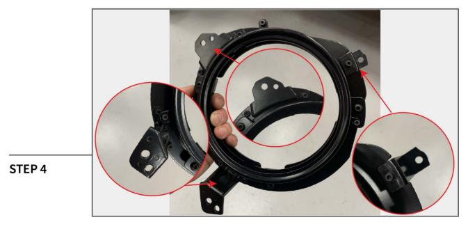
Starting on the Driver's side of the vehicle, locate all the brackets stamped "L". Using the provided Allen key and bolts assemble the LH bracket.
