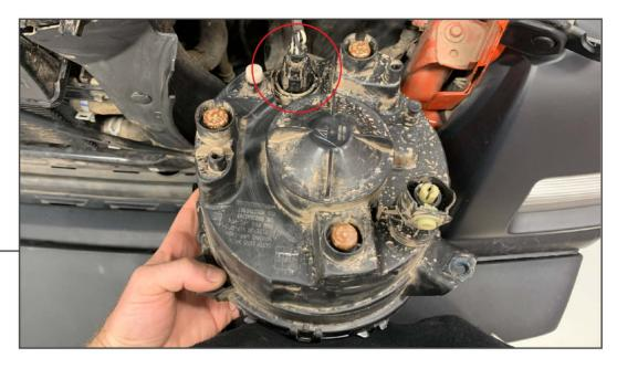
Pull the headlight away from the vehicle. Pull back the red plug locking tab, then depress the clip and pull the plug away from the light. Remove the light from the vehicle.
