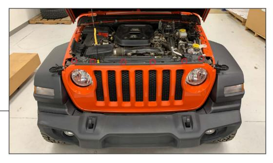
Begin by opening and supporting the hood. Use a soft pry tool to remove the (6) plastic push pins across the top of the grille. Then Firmly pull the grille away from the vehicle. Set the grille aside for re installation later.
