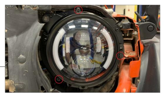
Remove the (3) Allen bolts using the supplier Allen key. Install the headlight retaining ring on any 7" headlight. Plug the light into the adapter harness and reinstall the (3) Allen Bolts. \*\*Note: 7" Headlights are NOT included.
