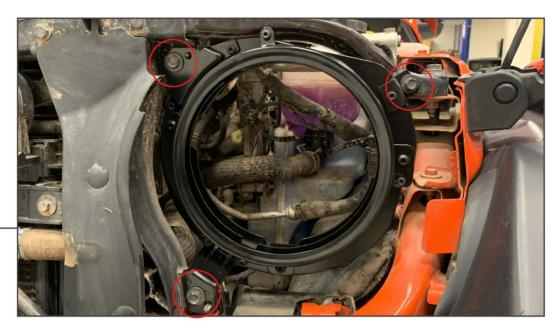
Install the adapter bracket to the vehicle using the factory hardware.
