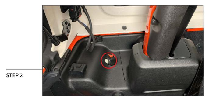
Using a 10mm socket, loosen the tail light retaining bolt.
