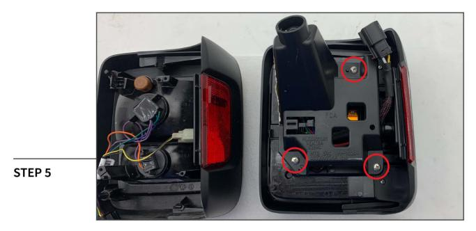
Screw the mounting bracket to the new light using the provided hardware.
