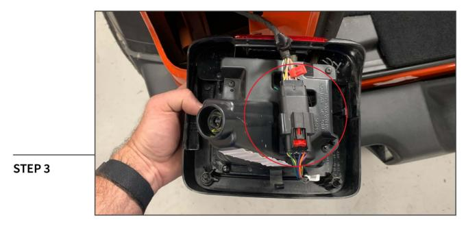
Pull the tail light away from the vehicle. Slide back the plug's red locking tab. Depress the connector and pull it away from the tail light. Disconnect any clips holding the wiring to the tail light.
