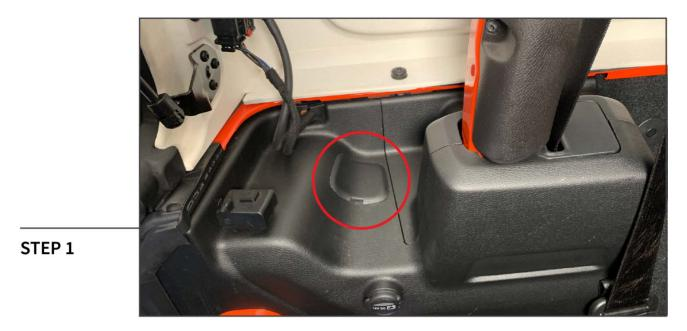
Begin by opening the tailgate to gain access to the tail light retaining bolt. Using a soft pry tool remove the trim panel.
