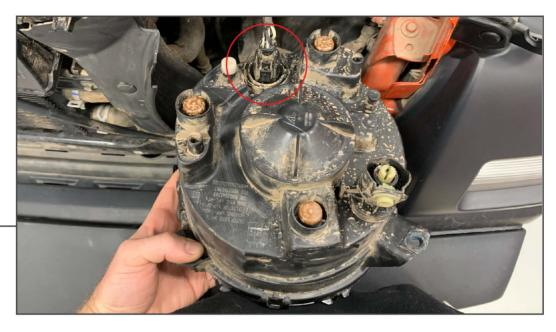
Pull the headlight away from the vehicle. Pull back the red locking tab, then depress the clip and pull the plug away from the light. Remove the light from the vehicle.
