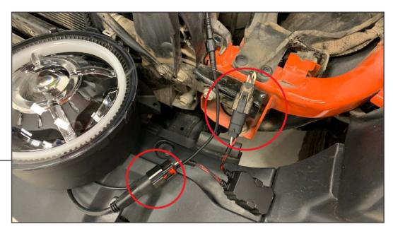
Plug the headlight harness into the vehicle and then into the headlight. Using the factory hardware, reinstall the headlights.
