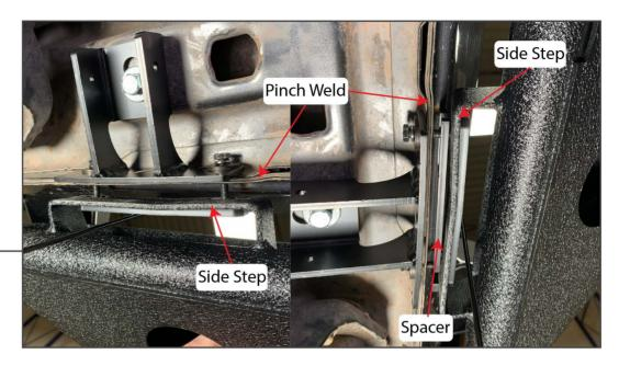
If the side step is too close to the body, install the supplied spacers between the side step and the pinch weld.
