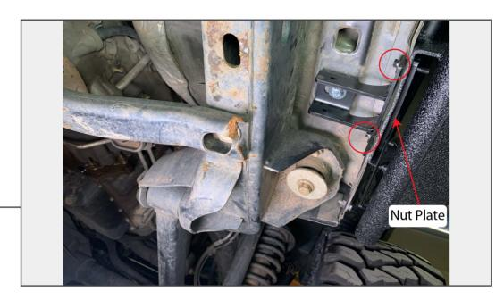
The larger step pad will be towards the front of the vehicle. With a helper, hold the side step to the vehicle. Loosely install (2) M6x1.00 Bolts, (2) M6 Lock Washers, (2) M6 Flat Washers, (1) Nut Plate on the front mounting location is shown above.
