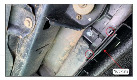
Loosely install (2) M6x1.00 Bolts, (2) M6 Lock Washers, (2) M6 Flat Washers, (1) Nut Plate on the rear mounting location is shown above.
