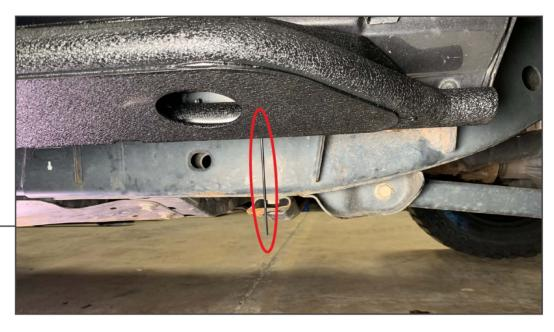
Adjust the steps side-to-side as needed. Then tighten all bolts. Remove the nut plate handle by bending the handle back and forth until it breaks off the nut plate.
