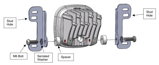
Step 4: Mount Squadrons onto the bumper with the 8 included plastic screws.
