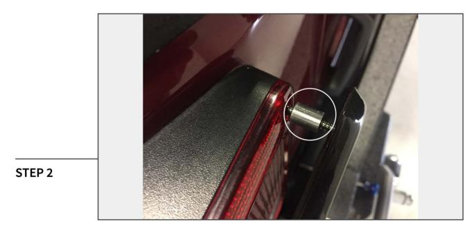
Install the spacers between the tail light and the tail light guard.
