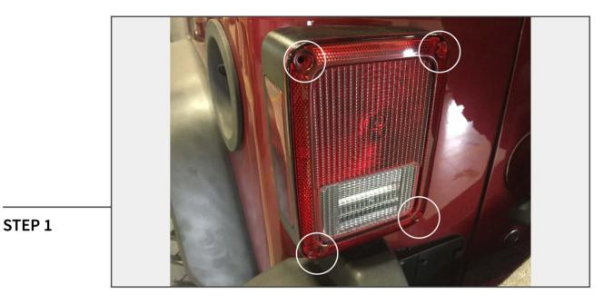
Using a Phillips head screw driver, remove the (4) screws on the tail light. Note: the location of the thick and thin screws.
