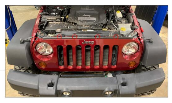
Using a soft pry tool, remove the (6) plastic push pins across the top of the factory grille cover. Then firmly pull the grille cover away from the vehicle. Disconnect the factory turn signal plugs. Slide back the red tab lock, then depress the tab and pull the plug away from the light.
