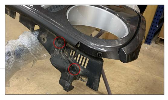
Using a soft pry tool, remove the foam corners from the factory grille and transfer them to the new grille.
