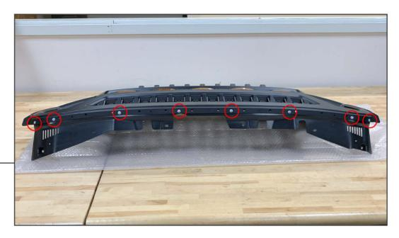
Using the supplied nuts, bolts, and washers attach the upper grille to grille cover.
