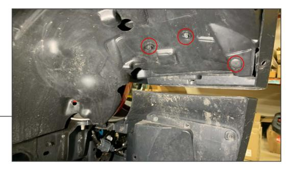
Fold back the fender liner to access the fender marker light wiring. Remove the (2) 8mm screws and (1) push clip.
