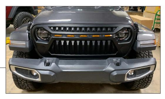
Reinstall the grille using the (6) plastic push clips. Install the supplied weather stripping across the top edge of the grille.
