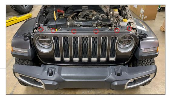
Using a soft pry tool, remove the (6) plastic push pins across the top of the factory grille cover. Then firmly pull the grille cover away from the vehicle.
