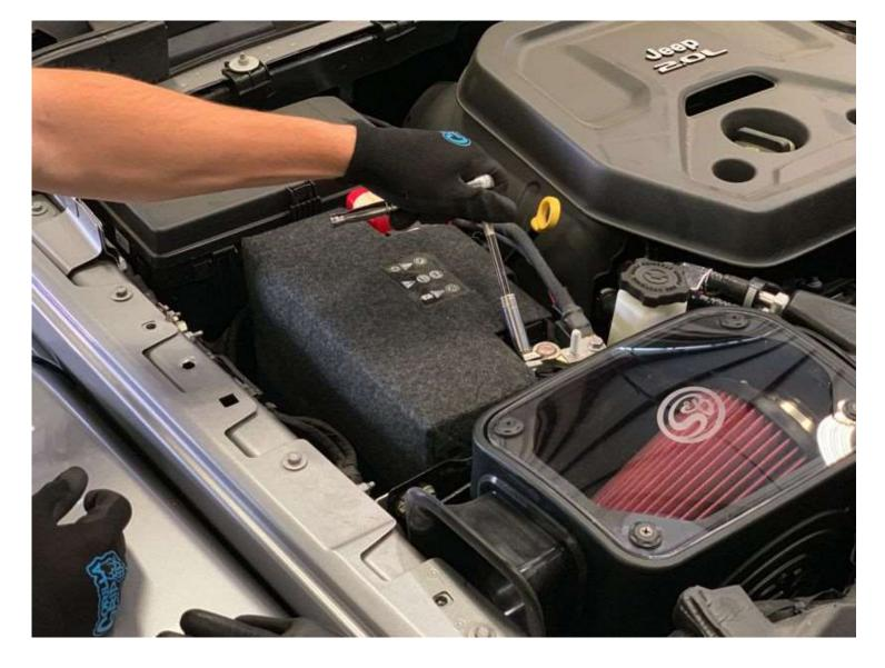
Reconnect the negative terminal on battery. Inspect your installation, make sure the kit is properly positioned and all fasteners are secured. S&B Filters recommends keeping all stock parts in case you would ever need to reinstall the stock intake.
