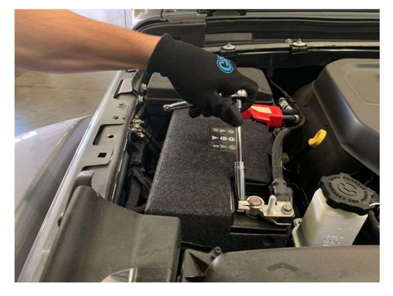
With the ignition switched off and the parking brake set. Disconnect the negative battery cable on the passenger side.
