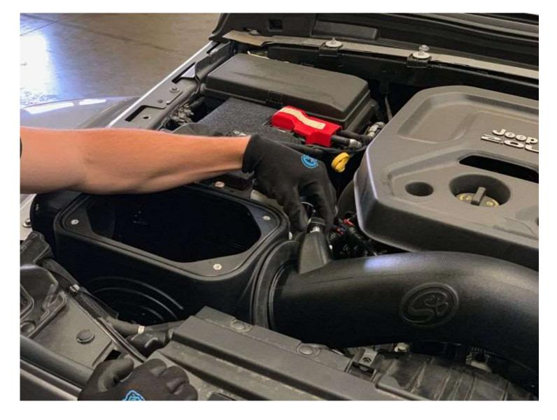
Reconnect the two EVAP tubes to the EVAP Fitting (Item I). There should be an audible click when the tubes are fully inserted.
