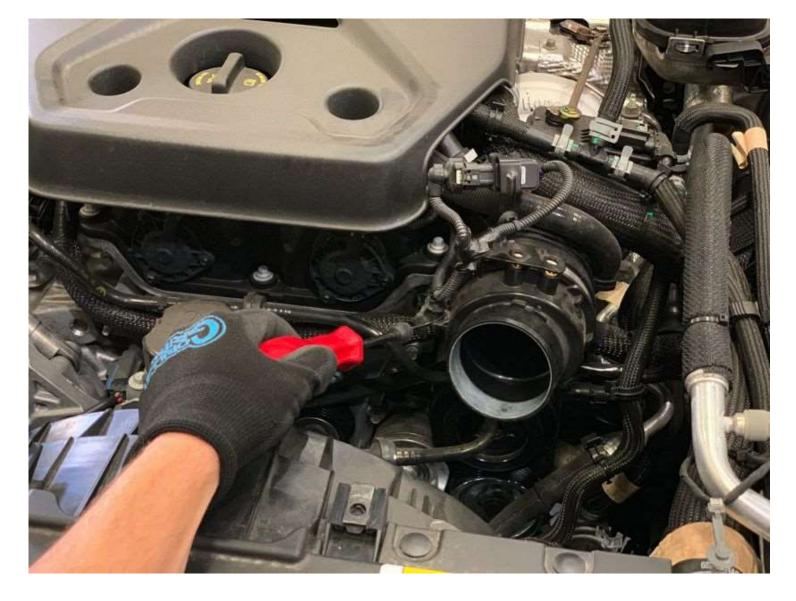
Disconnect the clip securing the wire harness to the turbo resonator.
