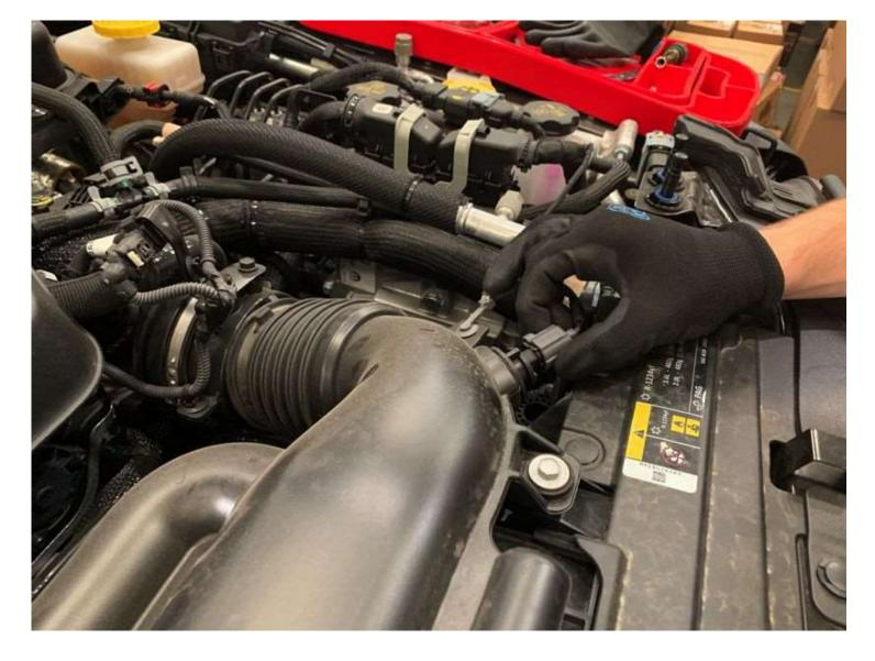
Disconnect the IAT electrical harness from the IAT sensor by pressing down on the locking tab and pulling off the IAT sensor connector.
