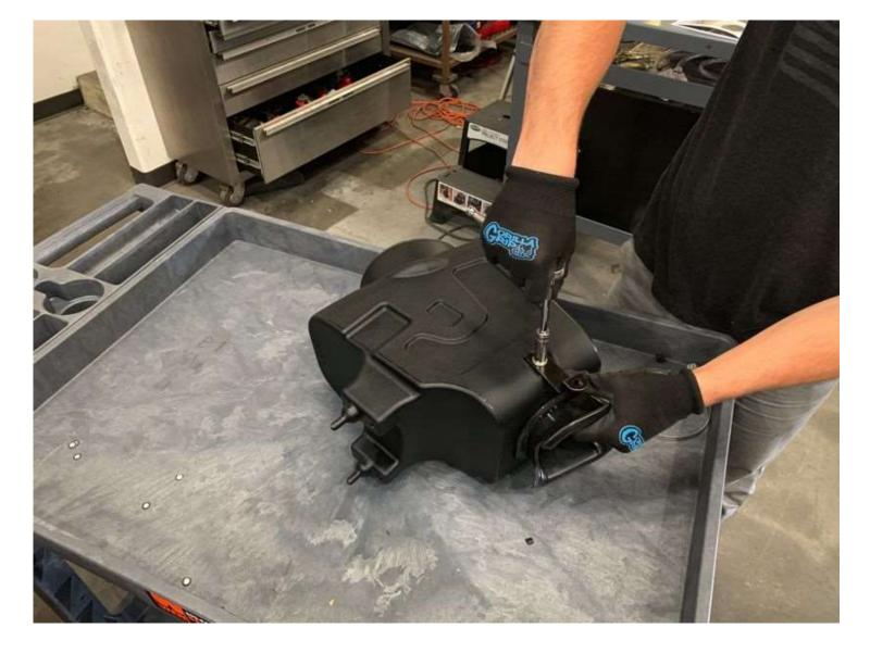
Install and tighten the Bracket (K) with the M6 Bolt (L) and M6 Washer (Q) onto the Intake Box (A). Do not overtighten.
