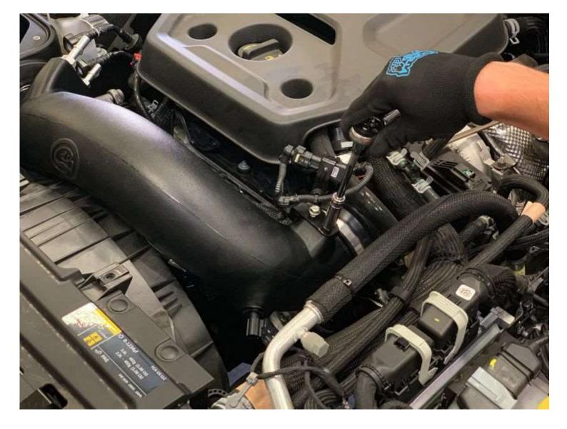
Install the wire harness bracket onto the Intake Tube (B) with the M6 Bolts (L).
