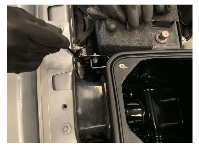
Position the Fender Seal (C) up against the fender then secure the Bracket (K) to the battery tray bracket with a supplied M6 Bolt (L). Do not overtighten.
