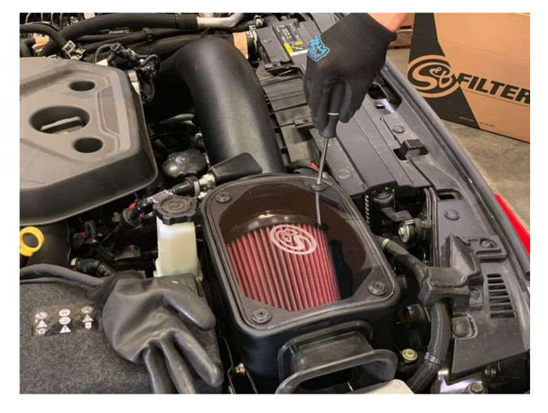
Place the Clear Lid (G) onto the Intake Box (A) then secure using the provided Lid Screws and Washer (O & P). Do not overtighten.
