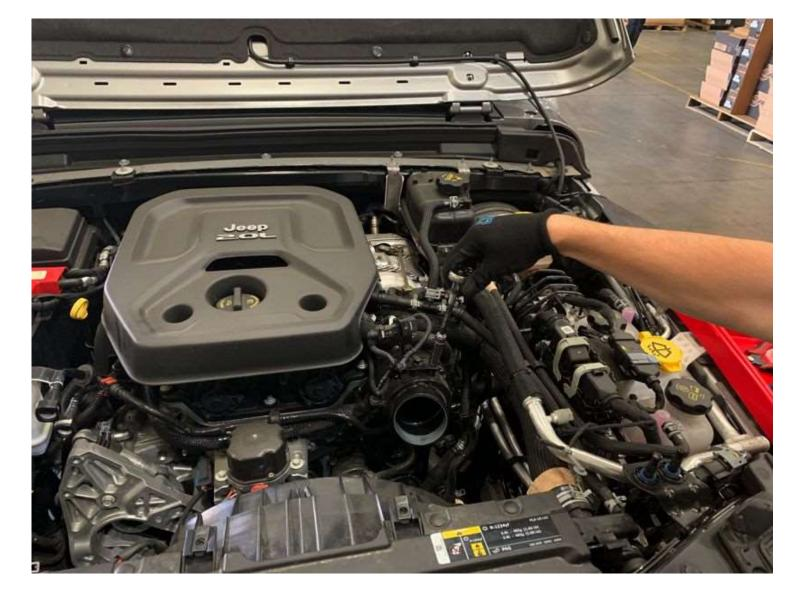
Remove the two bolts securing the wire harness bracket to the turbo resonator chamber.
