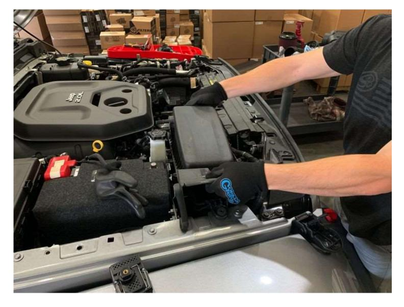
Lift the stock intake box to unseat the prongs from the grommets then remove the stock intake box from the vehicle.
