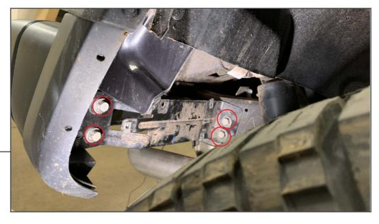
Behind the fender liners removed in Step 2, remove the (4) 16mm bumper brace bolts on both sides of the bumper.
