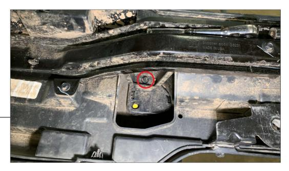
Using a 7mm socket, remove the screw securing the factory reflector to the vehicle. Then press the reflector out of the bumper.
