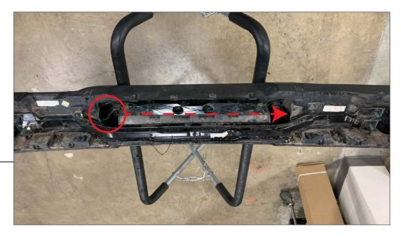
Route the wiring from the RH light over to the LH light.
