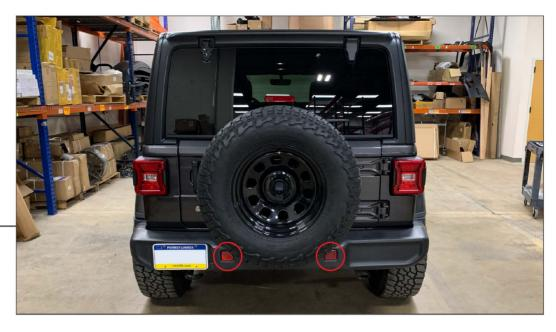
For this install, you will need access to the back of the factory reflectors. To do so removal of the bumper will be required.
