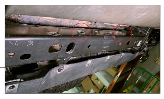
Remove the (2) 18mm bolts securing the center of the bumper to the vehicle.
