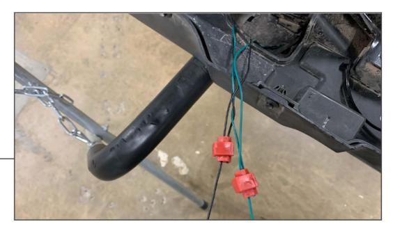
Using the (2) of the supplied Scotchlok connectors, join the RH light and LH light wiring together.
