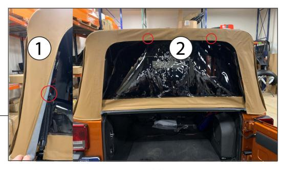
Unzip the left hand side of the slider half way up the window(1). Then, align the sliders 12" apart on the top of the window. Doing it this way will put less stress on the zipper and window components.
