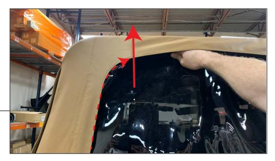
Align the zipper halves on the rear window and the top. Gently start pulling the slider around the window. Take special care around the first corner, pull up on the window as you pull the zipper around the corner. Once the rear window is zipped half way(center of the window) STOP.
