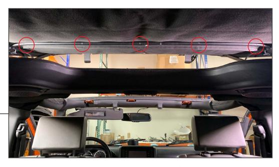
Fold the top back to gain access to the screws securing the top to the frame/hardware. Remove the (5) Phillips head screws securing the top to the front bow. The screws will be reused during re installation.
