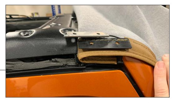
Install the header sandwich plate. Install the screws working from the center out. Carefully tuck the corner of the top into the header plate.
