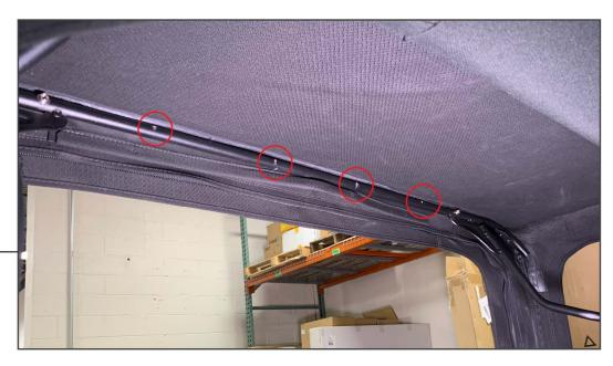
Next, remove the (4) screws that hold the top to the rear bow. The screws will be reused during re installation.
