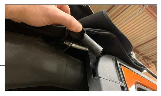
Disconnect the cables from the frame/hardware. Gently fold back the plastic cover and unhook the spring.
