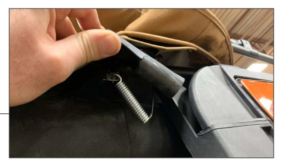
Feed the tensioning spring through the plastic shroud. Using pliers, attach the spring to the frame/hardware.
