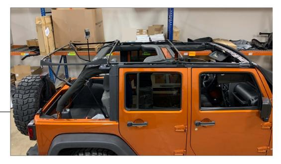
Start by confirming that your vehicle has the factory soft top frame/hardware. If your vehicle does not you will need to purchase a factory frame/hardware for this installation. Vehicles that came with a factory hardtop typically do not have the factory frame/hardware.
