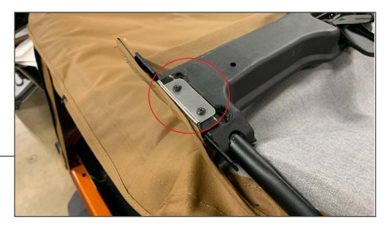
Fold the front of the top back. Secure the tensioning cable anchor to the header using the original hardware.
