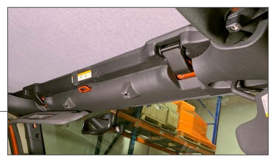
Secure the header to the vehicle by reconnecting the factory hooks to the windshield frame. Then push down on the latch to secure it to the vehicle. New tops are normally tighter and may require more effort when pulling them down onto the windshield.
