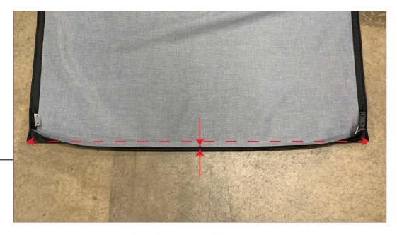
Using a tape measure, measure the width of the front edge of the top. On the underside of the new top, mark the center line.
