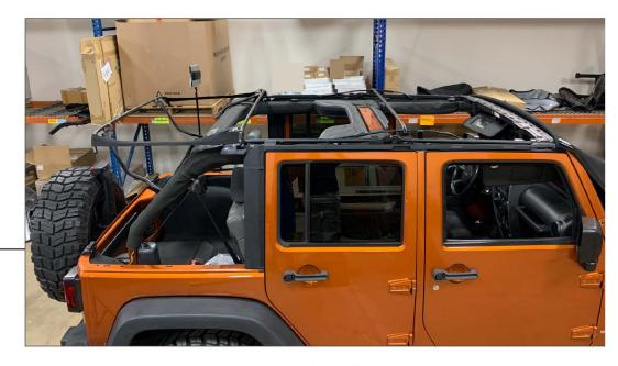
Start by confirming that your vehicle has the factory soft top frame/hardware. If your vehicle does not you will need to purchase a factory frame/hardware for this installation. Vehicles that came with a factory hardtop typically do not have the factory frame/hardware.
