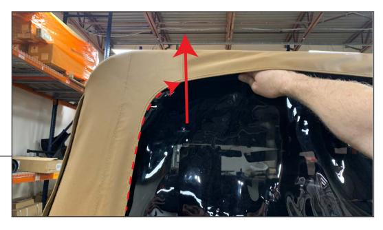
Align the zipper halves on the rear window and the top. Gently start pulling the slider around the window. Take special care around the first corner, pull up on the window as you pull the zipper around the corner. Once the rear window is zipped half way(center of the window) STOP.
