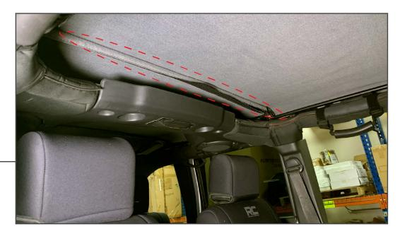
Wrap the top around the forward most bow and secure the top to itself using the hook and loop.
