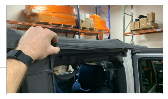
Unhook the top from around the window channels.
