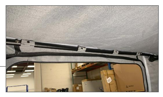
Secure the top to the rear bow using the original hardware. The fabric mounting tabs do not come with pre-drilled holes. Carefully screw the factory hardware through the fabric tabs into the metal bow.
