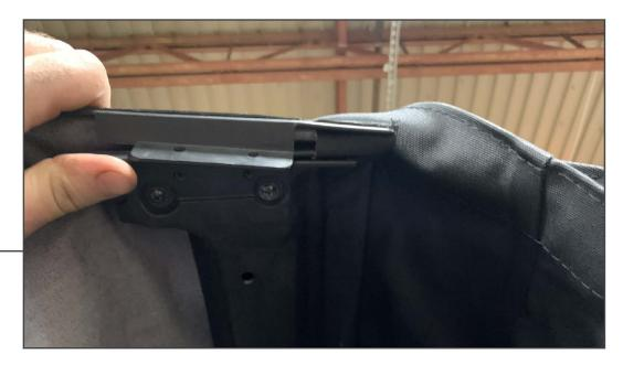
Install the header sandwich plate. Install the screws working from the center out. Carefully tuck the corner of the top into the header plate.
