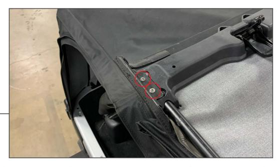
With the top half down, remove the (2) screws that hold the front edge of the top to the sides of the headers. These will be reused during re installation.
