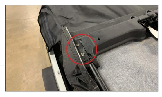
Fold the front of the top back. Secure the edge to the header using the screws removed in Step 9.
