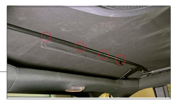
Remove the (4) Phillips head screws securing the top to the center bow. The screws will be reused during re installation.
