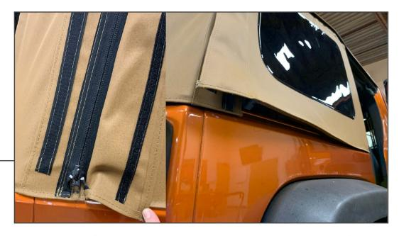
Zip the zipper to the bottom rear of the window. Fasten the hook and loop over the top of the rear window. Then tuck the bottom edge of the window under the retaining lip on the rear of the vehicle.
