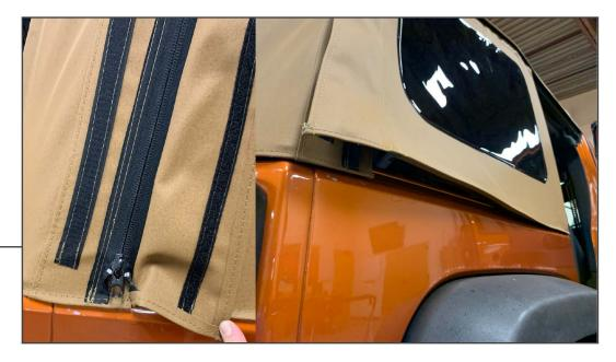
Zip the zipper to the bottom rear of the window. Fasten the hook and loop over the top of the rear window. Then tuck the bottom edge of the window under the retaining lip on the rear of the vehicle.
