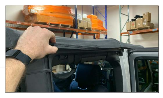
Unhook the top from around the window channels.
