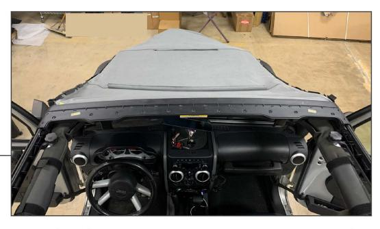
Fold the entire top over the front of the vehicle to access the header. The header clamps the front edge of the top onto the frame/hardware. There are (27) screws, carefully remove all the screws, keep note of what screws go where as there are (2) different length screws.
