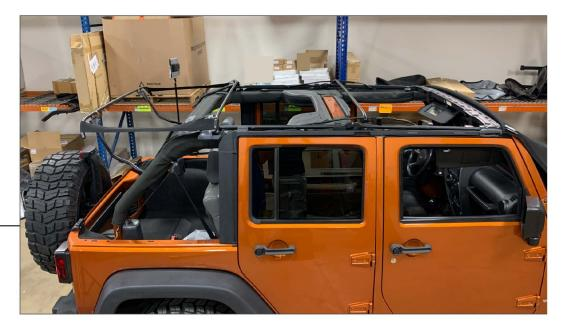
Start by confirming that your vehicle has the factory soft top frame/hardware. If your vehicle does not you will need to purchase a factory frame/hardware for this installation. Vehicles that came with a factory hardtop typically do not have the factory frame/hardware. Photos are for demonstration purposes, 2 door and 4 door tops install in the same fashion.
