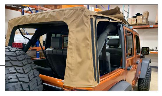
Secure the rear corners to the vehicle by tucking the plastic under the retaining lip on the rear of the vehicle.
