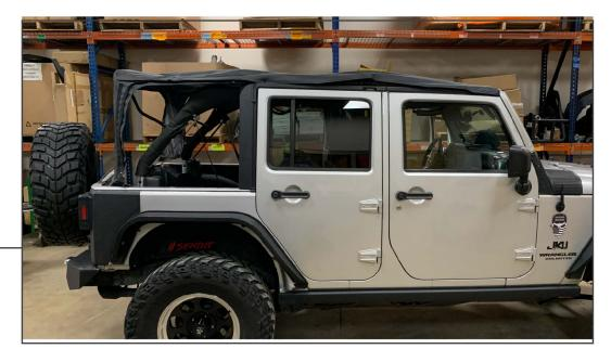
Fold the top back over the windshield onto the factory frame/hardware.
