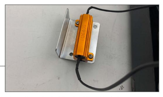
Using a Phillips head screwdriver and a pair of pliers, install the resistors to the resistor mounting bracket. Each resistor will require (2) machine screws and (2) lock nuts.
