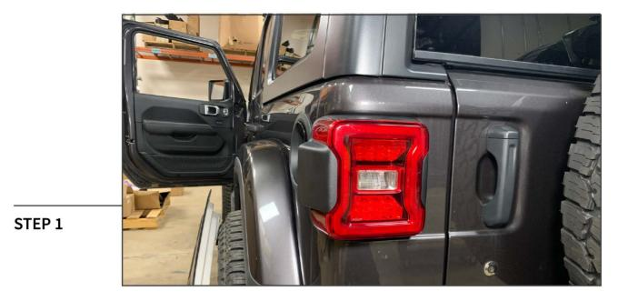
Begin by thoroughly cleaning the tail lights. Use rubbing alcohol to remove any remaining wax and grease. Allow the light plenty of time to dry. The double sided tape will not stick if the lights are wet.
