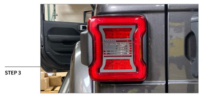
Center the covers on the lights. Apply firm even pressure to the taped surfaces to ensure proper adhesion. Installation is now complete.
