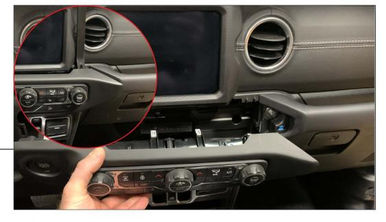
Using the provided soft pry tool, carefully pry the HVAC control panel away from the vehicle.
