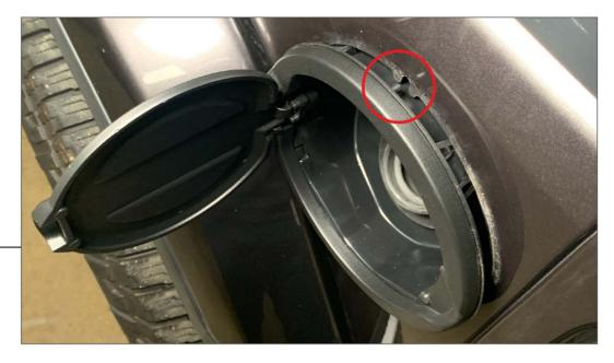
Alight the locating tab on the new fuel door with the vehicle. Carefully press the new fuel door over the fuel filler neck and on to the vehicle. Ensure it clips into place.
