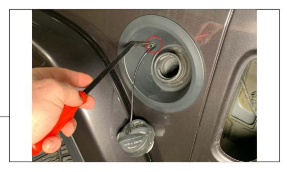
Remove the fuel cap from the filler neck. Then using a soft pry tool, remove the cap's tether
