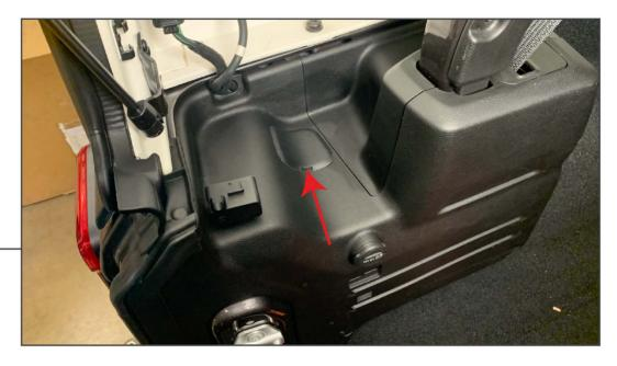
Begin by opening the tailgate to access tail light trim cover. Using a soft pry tool, remove the cover.
