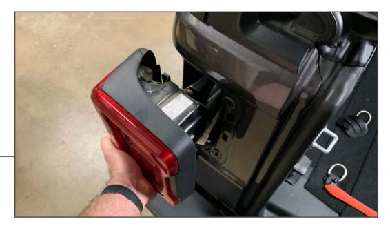
Pull the tail light away from the vehicle to access the light's wiring connection.
