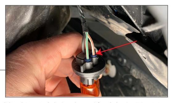
Turn the running light socket counter clock-wise and remove it from the housing. Using a test light, turn on the running lights and test for 12v+ power at the plug. On this vehicle the white/brown wire is the DRL wire. Connect the provided yellow wiring harness to the white/brown wire. Run the spade end of the wire to the headlight bucket.
