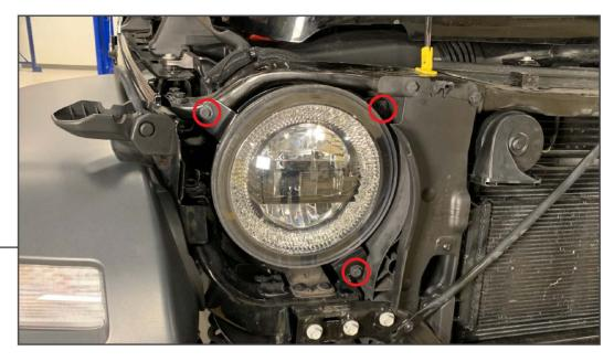
Install the LED headlight onto the vehicle using the factory hardware. Test the lights for functionality and alignment.
