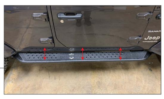
Next, determine if your vehicle will require any additional spacers. Carefully hold the side step the pinch welds of the vehicle. If the gap is consistent between the slider and the body of the vehicle you will not need to use spacers. If the slider gap is inconsistent, use the included spacers to create the desired gap.
