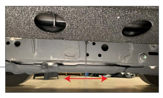
Once the side steps are bolted on, the nut plate holding rod is no longer necessary. Bend the rod back and forth. The rod will break off the plate. Discard the rod. Complete installation by torquing all fasteners following the chart below.
