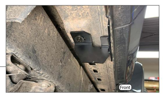
Using (1) M8x1.25 35mm bolt, M8 lock washer, and M8 flat washer loosely mount the middle pinch weld bracket to the vehicle.
