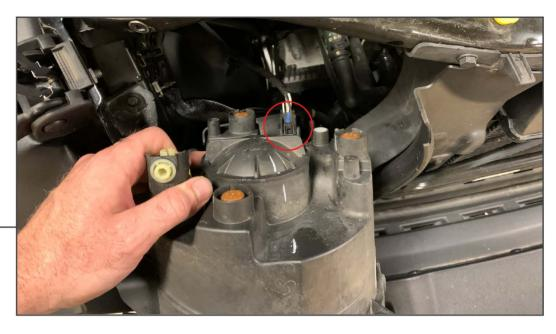
Pull the headlight away from the vehicle to access the wiring connection. Depress the tab and pull the plug away from the headlight.
