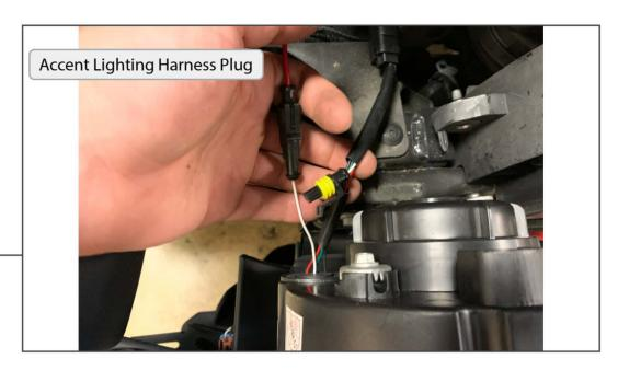
Unplug the white wire from the headlight harness and connect it to the accent lighting harness installed in step 4.
