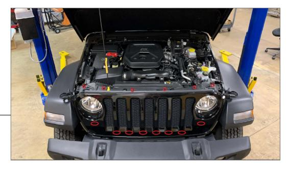
Begin by raising and supporting the hood. Remove the (6) plastic push clips that secure the grille to the vehicle. Then firmly pull the grille away from the vehicle to dislodge the (8) blind clips across the bottom of the grille and below the headlights.
