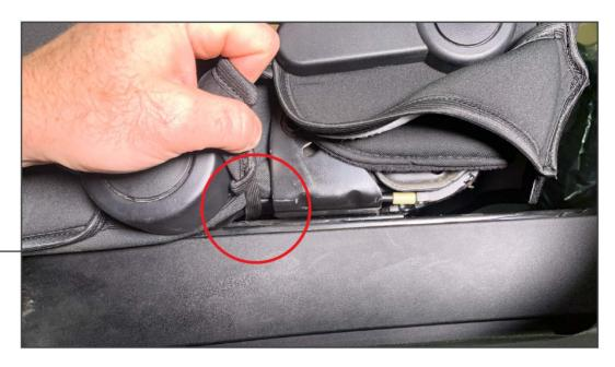
Route the side straps under the seat by feeding them through the gap below the seat bracket and above the slider. Location will vary from side to side, its not extremely critical but you just don't want the slider cutting the strap.
