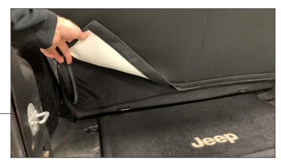
Continue to pull the soft portion of the cover from step 14 around the seat back. Attach the soft portion of the seat cover to the Velcro on the underside of the seat cover.
