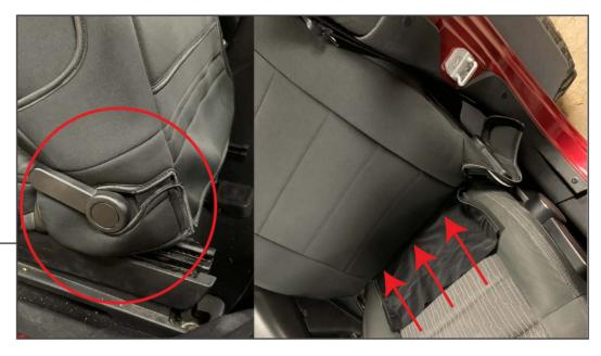
Wrap the upper cover around the seat lever and Velcro it to itself. Wrap the soft portion of the upper seat cover through the seat back. Folding the seat forward allows for more space between the seat back and seat bottom.
