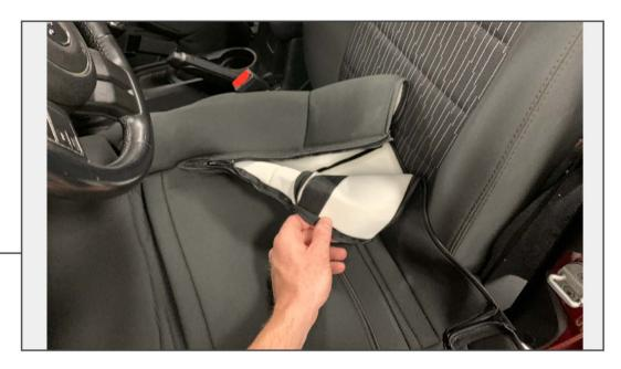
Locate the zipper on the back of the upper seat cover, this is the console side of the cover. Unzip the zipper to make the installation easier.
