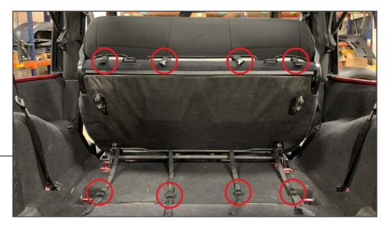
Position the lower portion of the seat cover over the seat bottom. Feed the straps towards the rear of the seat. Ensure the clips are pushed through the back of the seat.
