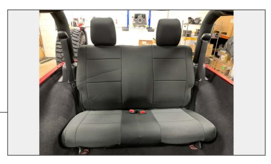
Reinstall the headrest and pull the seat belt receivers through the cover to complete the installation.
