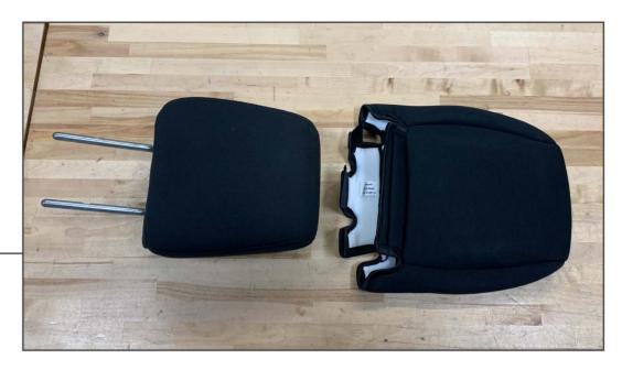
Install the headrest cover over the factory headrest. The tag on the cover will face the rear of the vehicle. Velcro the center together and then tuck the sides of the headrest cover under the center.
