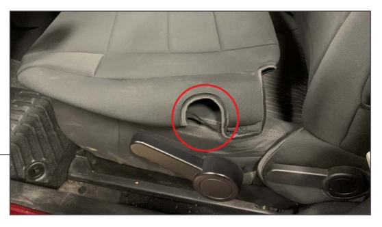
Identify the driver side lower seat cover by locating the hole for the seat height adjuster.
