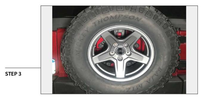
Remove the spare wheel center cap, then reinstall wheel onto the carrier, with the license plate base plate in the middle. Reinstall and tighten lug nuts to OE specifications (80 ft-lbs).
