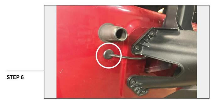
Route the wiring behind the spare tire mount, and route the wiring into the factory grommet in the tailgate for the 3rd tail light.
