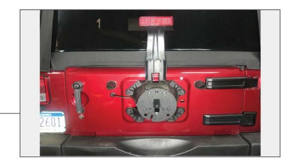
Using the provided base plate, place the plate over the factory carrier lug studs.
