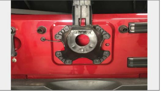
Begin by removing the spare tire. Using a 21mm socket and a breaker bar removed the (3) lug
