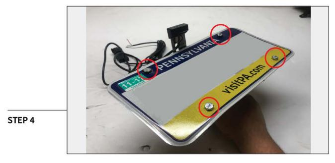
Attach the license plate light and the license plate to the mounting plate by using (4) M6x1.00 20mm bolts, and (4) M6 lock nuts.
